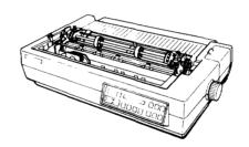
1. Press the tabs on the pull tractor. Then tilt the tractor back and lift it off the printer.
